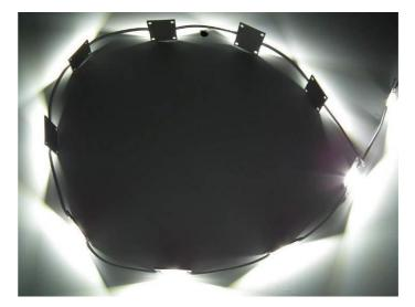
With secondary optical lens on LED, the emitting angle can be widened so that the light bar presents excellent light uniformity
